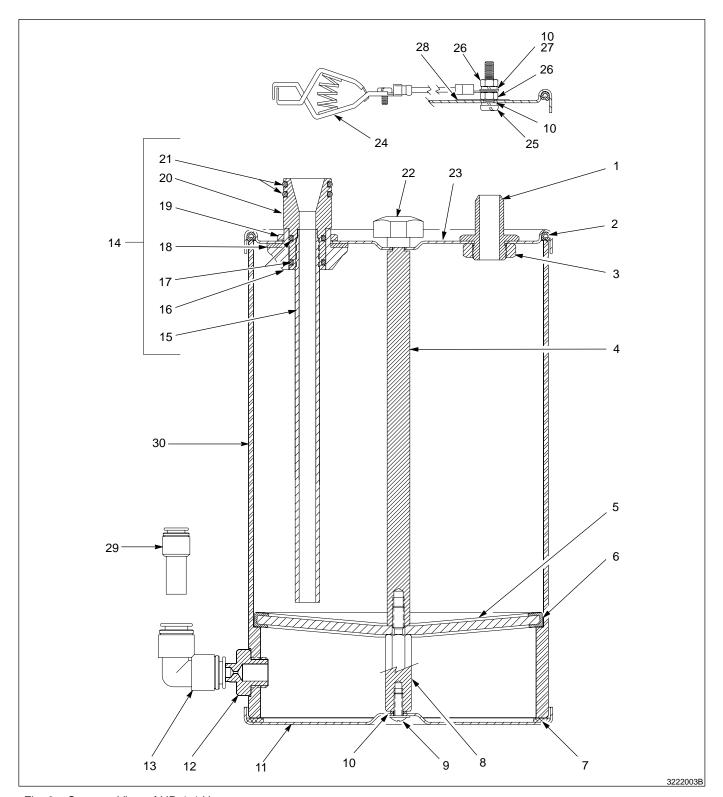
Fig. 3 Cutaway View of HR-1-4 Hopper
