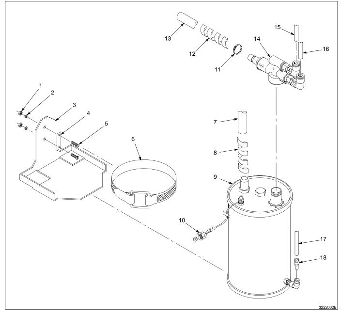
Fig. 2 Installing HR-1-4 Hopper
